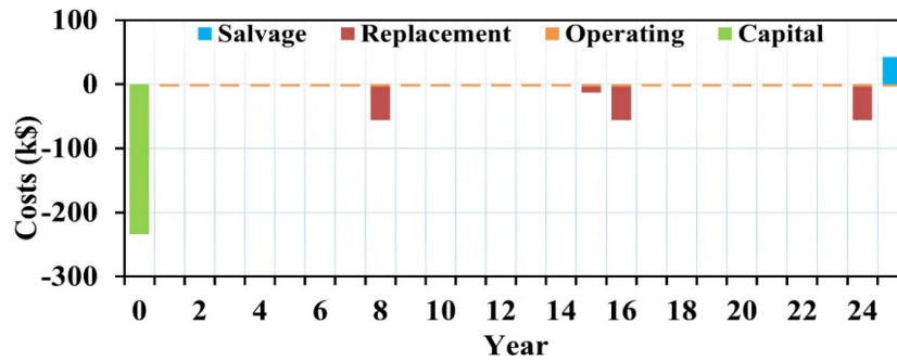
Fig. S15. Cash flow of PV, BAT, and CONV systems by cost type.
