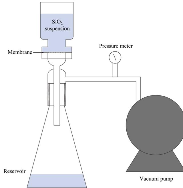
Fig. S2. Schematic of the dead-end filtration system.
