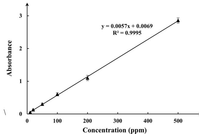
Fig. S3. The standard calibration curve of SiO<sub>2</sub> suspension.
