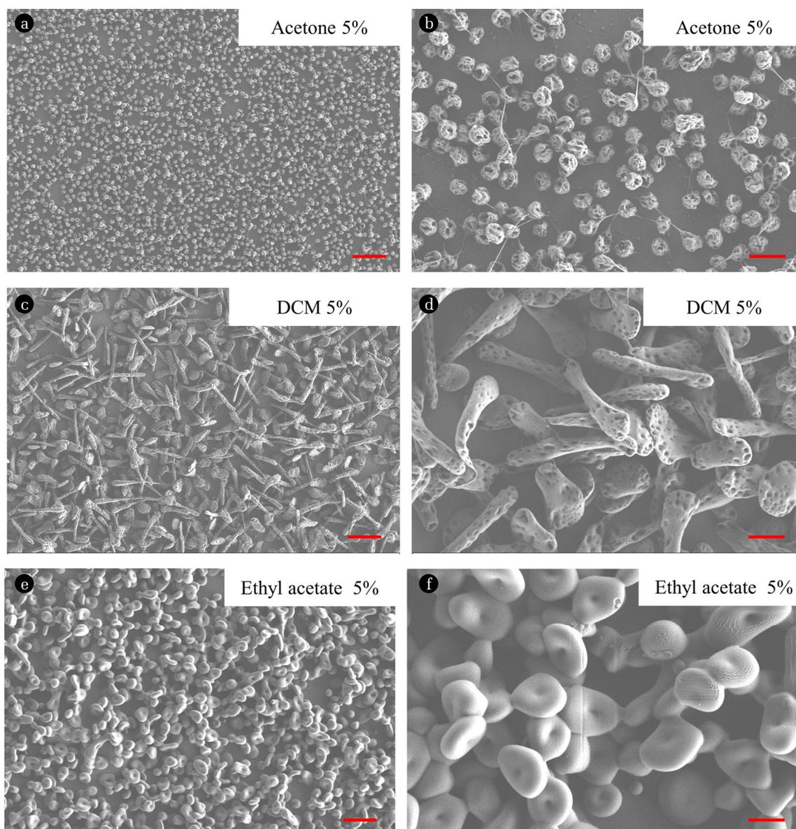
**Fig. S4.** (a), (c), (e) Various morphologies of microparticles fabricated with electrospray using different solutions. Scale bar: 20  $\mu\text{m}$ . (b), (d), (f) Zoomed-in SEM images corresponding to (a), (c), (e). Scale bar: 5  $\mu\text{m}$ .
