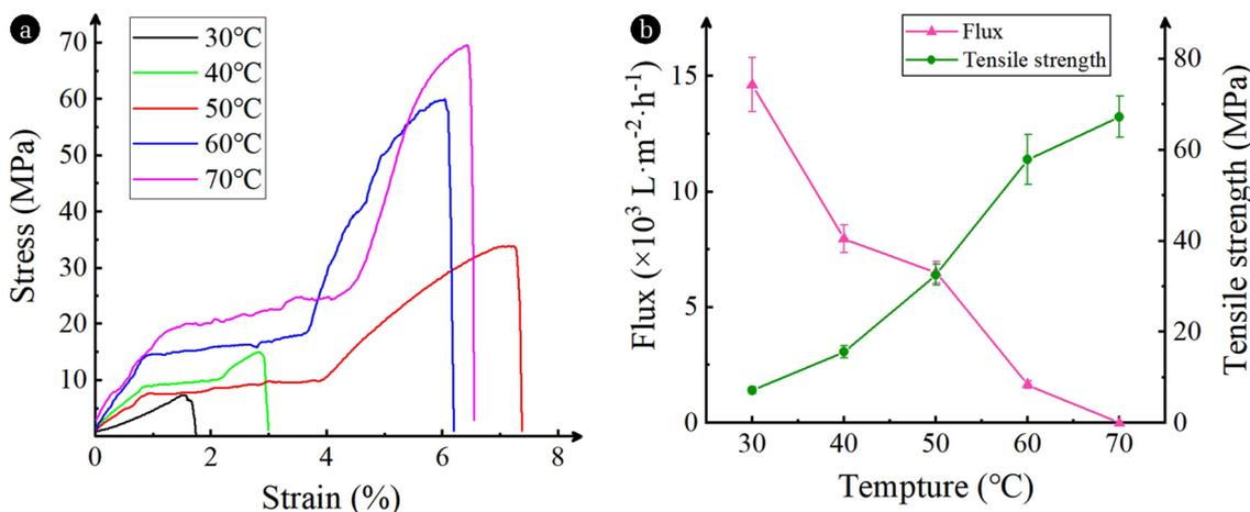
**Fig. S1.** (a) The stress-strain curve of particulate membranes after thermal treatment at different temperatures. (b) The pure water flux and tensile strength of particulate membranes after thermal treatment at different temperatures.
