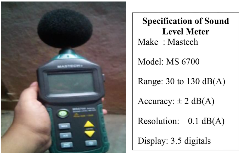
Fig. S3. Sound level meter used in this study to collect noise data
