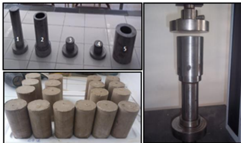
Fig. S2. Device used for the preparation of samples (50X100) mm.
